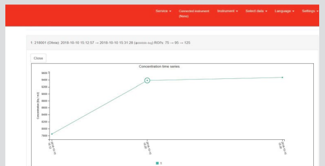
Time distribution for 18 min sniffing at 9400 Bq/m 3 . After 8 min, ATMOS shows > 90% of true value.
